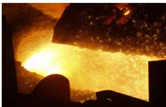
Fig. 1. Abnormal duration splashing during iron tapping at CSC's No.2 blast furnace.
